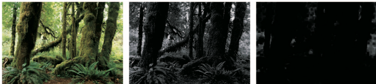
(L) \mathbf{J} ; (M) For each \mathbf{x} , minimum of its (R, G, B) values; (R) I^{\text{dark}} .
