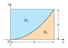
Solution. The parabola with vertex at (0,0) and passing through (a,b) is  $y = f(x) = \frac{b}{a^2}x^2$ . Then the centroid of  $\mathscr{R}_1$  is given by
